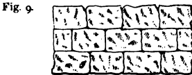
Fig. 9. Block Coursed. —Large blocks in courses (regular or irregular), Beds and Joints roughly dressed.
